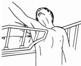
Entrapment between split bed rails
