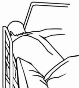
Entrapment between the end of the rail and the side edge of the head board or foot board
