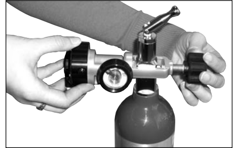
FIGURE D Attaching the BONSAI® Conservers to the Cylinder (Model OM-800 shown)
